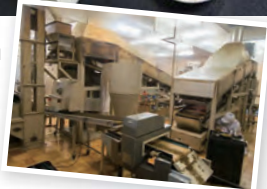
▶ Lightly roasted with far infrared radiant heat.
